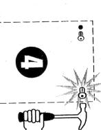
Insert anchors into holes and tap in place.
