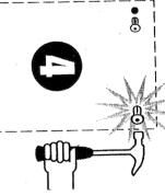
Place frame against the wall, line the mounting holes up with the anchors and screw in place.
